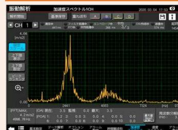
The system constantly monitors troubles in the equipment by analyzing vibration sensor and other data. Alarm appears on the screen in troubles.
