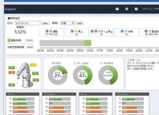
Equipment operation and consumables status can be checked on the cloud screen. HirataFE connects remotely to determine the cause of the problems and provide restoration support.
